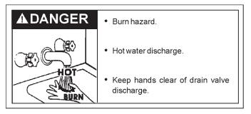
4. Attach a hose to the water heater drain valve and put the other end in a floor drain or outdoors. Open the water heater drain valve. Open a nearby hot water faucet which will relieve pressure in the water heater and speed draining. The water passing out of the drain valve may be extremely hot. To avoid being scalded, make sure all connections are tight and that the water flow is directed away from any person, see Figures 1 and 4.
